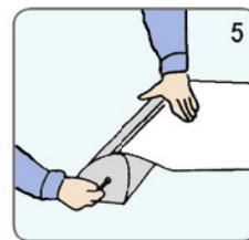
Hold the graphic and the roll-up body with one hand tight. Take out the pin at the side while you still hold the graphic, to avoid that graphic suddenly roll into the body too fast.
