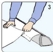
Take the protective film of the adhesive tape. Place the graphic evenly on the leading paper. Use the line as a guideline.
