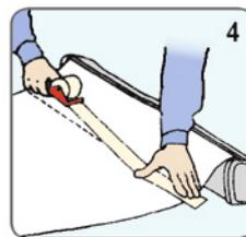
Put adhesive tape on the back of the graphic and on the leading paper, in order to secure the graphic to the leading paper.
