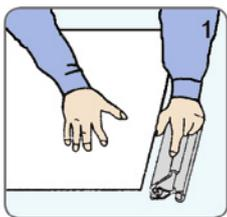
Open the snap clip, insert the top of the graphic into the gap, make the graphic flat.
